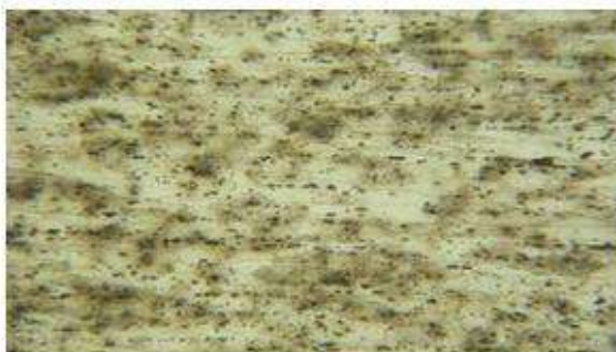
Gambar 9: struktur mikro lokasi 1 area material dasar (BM), perbesaran 100 x
