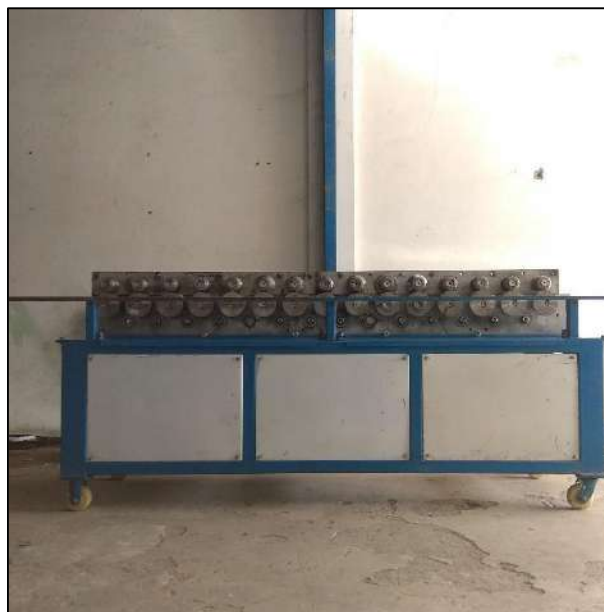
Gambar 5 Hasil Perakitan Mesin Transverse Ducting Flange (TDF)
