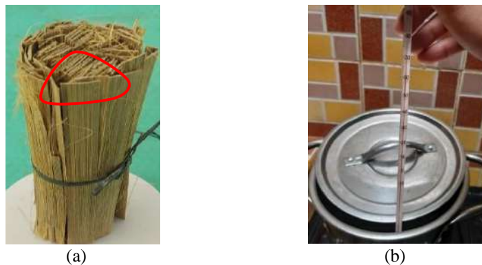
Gambar 1 (a) Daging bambu; (b) Proses perebusan daging bambu dan pengontrolan suhu 70°C [22]
