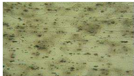
Gambar 10: struktur mikro lokasi 1 area material dasar (BM), perbesaran 200 x
