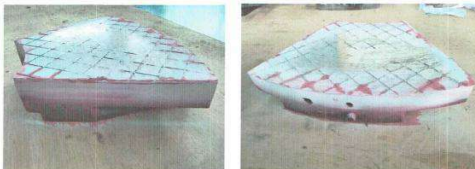
Gambar 3. Pad thrust bearing (terkikis)
