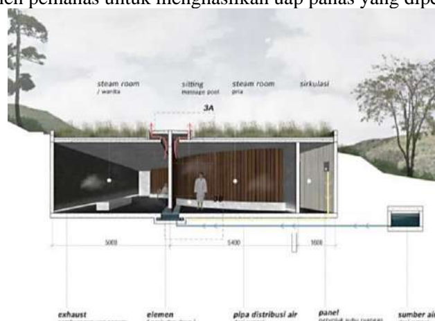
Gambar 7. Potongan Perspektif Steam Room.
