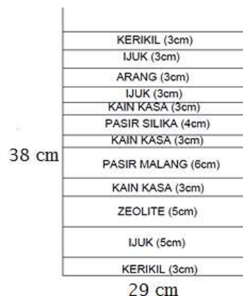
Gambar 2. Susunan Media Filter
