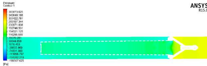
Gambar 7 Simulasi Hasil Pressure Drop Desain Original ( pressure contour )
